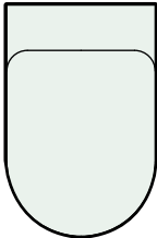
Quantum Square Wall Hung WC W360 x D560 x H340mm Height From Floor 410mm
